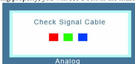
This box appears during normal operation if the video cable becomes disconnected or damaged.
